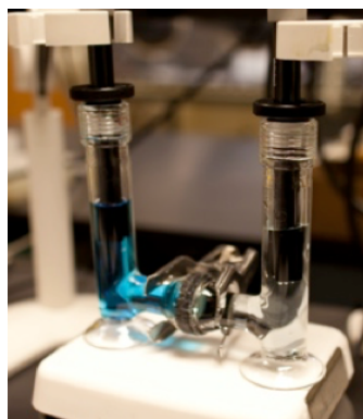
Fig. 2.1: Experiment to determine crossover rate of \text{VOSO}_4 through Celgard membrane.
