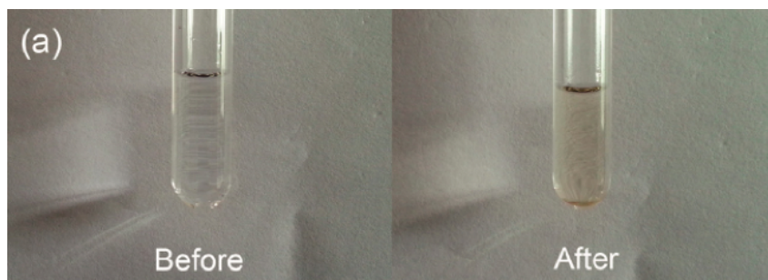
Fig. 4.5: 1 M \text{LiPF}_6 solutions: (left) solution that had been stored in a vacuum-dried aluminum bottle; (right) solution stored in an air-dried aluminum bottle.
