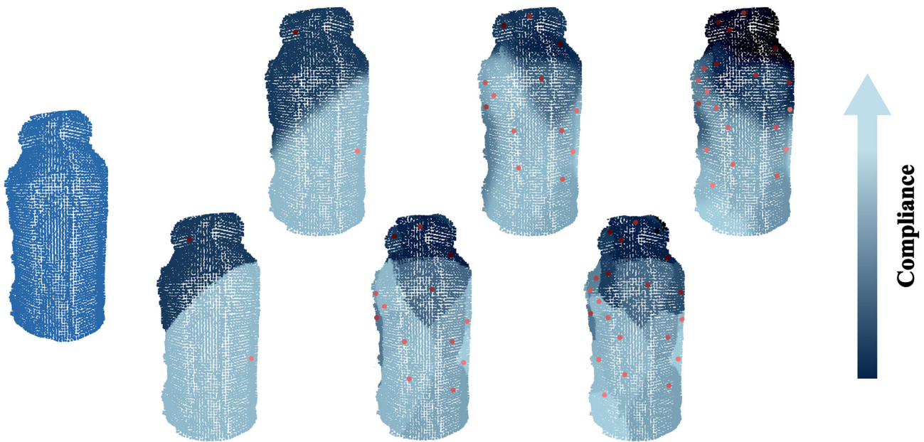
Fig. 2 Augmented PC representation at different number of touches. Starting from the visual PC (left), i.e., no tactile information, the colormap is updated by increasing the number of touches, thus obtaining a more accurate representation of how the compliance varies across the
