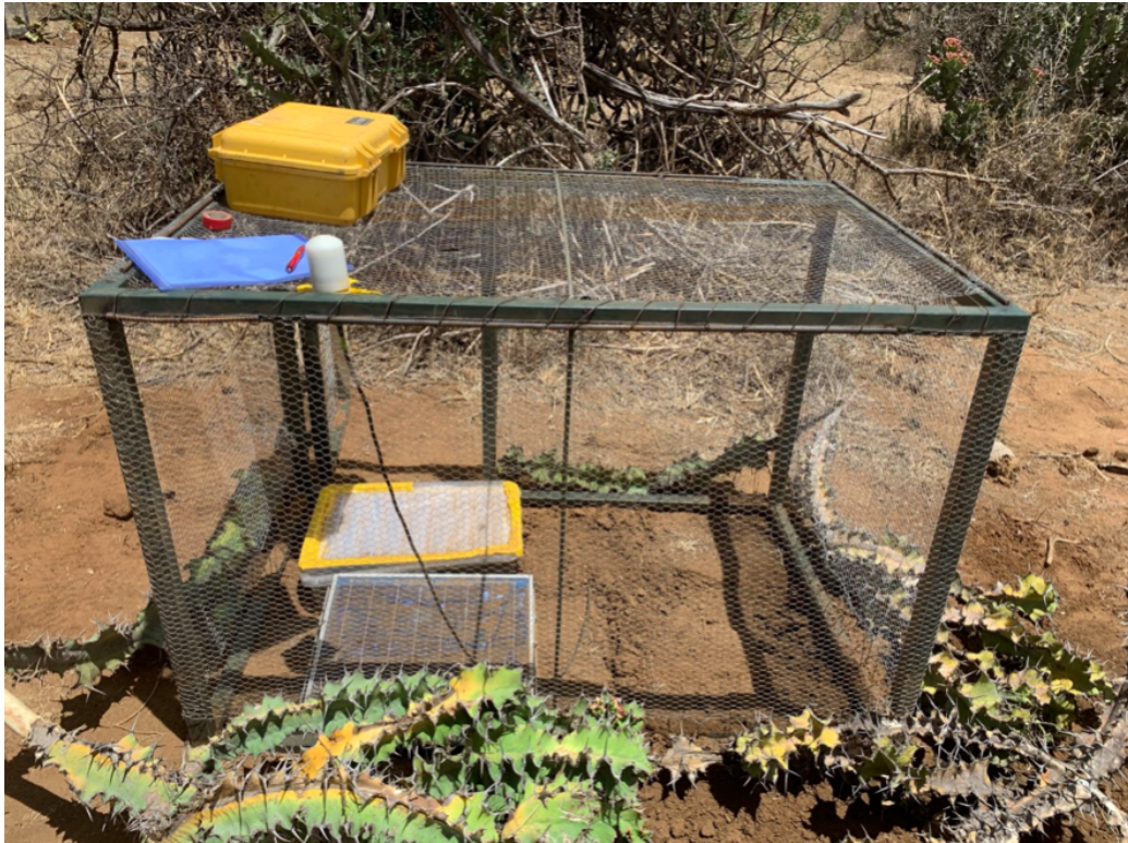
Figure 2.1: A deployed seismometer. The instrument is buried inside a cage to protect it from animals.
