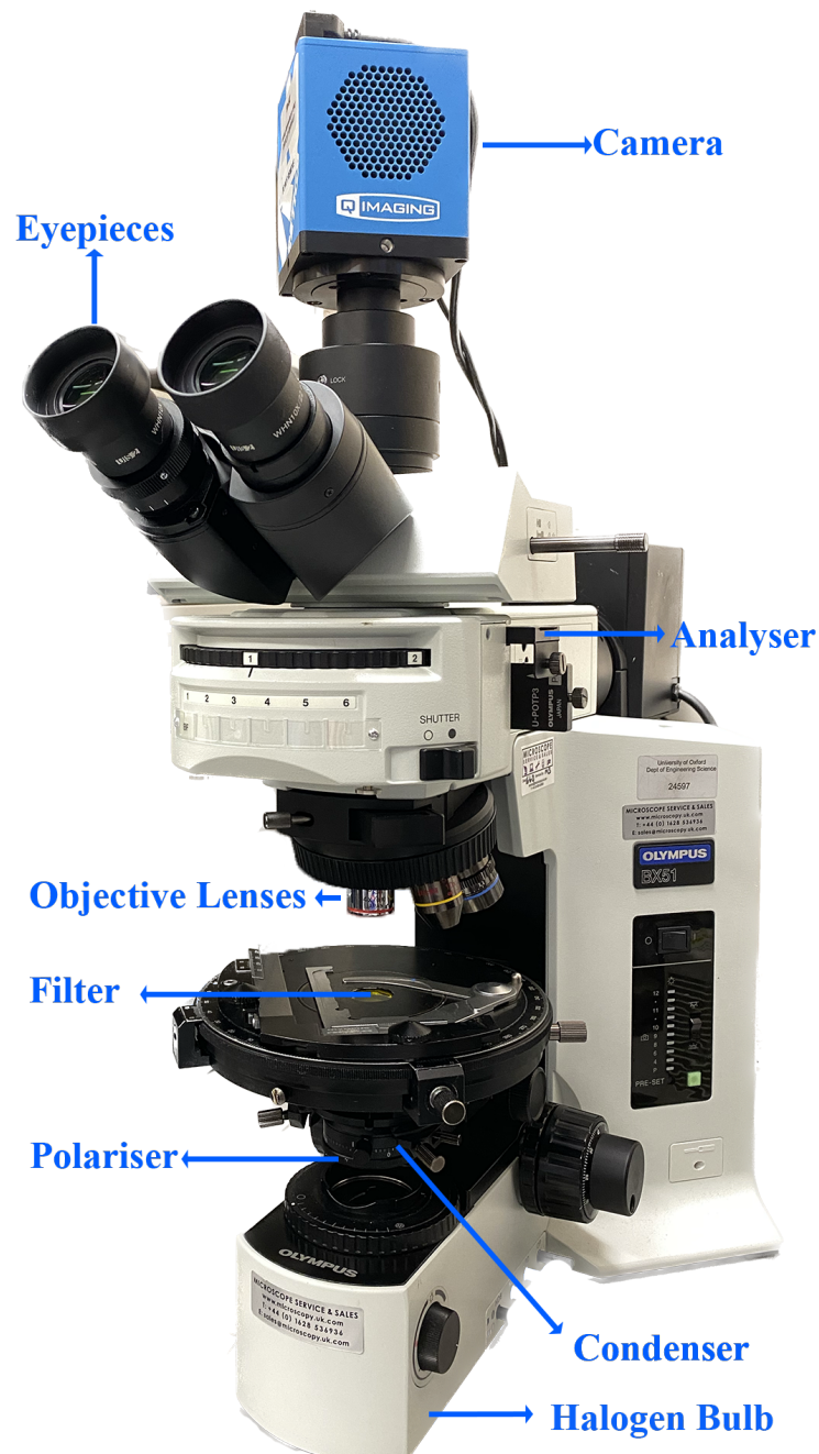
FIGURE 3.4: A photograph of the BX51 Olympus microscope and QImaging camera used in this thesis.
