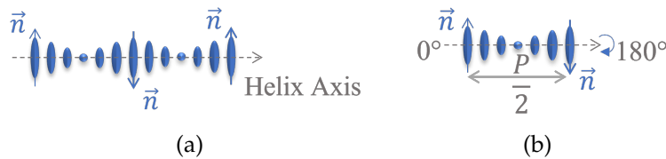
FIGURE 2.2: Molecules in a chiral nematic LC (cholesteric) phase. (a) shows the macroscopic configuration of the director of a chiral nematic LC phase. The orientations of the specific molecules are given by the director \vec{n} . The grey dashed line in (a) and (b) represents the helical axis of the chiral structure. (b) illustrates half of the pitch within which the director gradually rotates from 0 to \pi .
