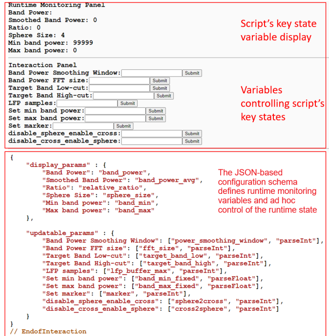
Fig. 4. A zoom-in view of the JSON-based configuration schema and the runtime monitoring and control panel.
