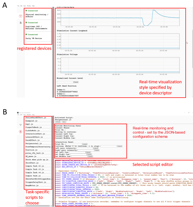
Fig. 3. Main views of the control-side program developed with Electron. A , Left panel: list of registered devices. Right panel: real-time visualization of report data. B , Left panel: Task-specific control scripts available to choose. Right panel: top, script management (activate and save), middle, script state variable visualization and control, bottom, script editor.
