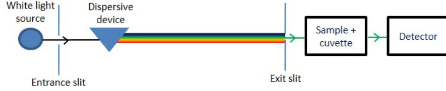
FIGURE 4.3: Schematic of the Cary 5000 UV-Vis-NIR spectrometer. A white light source is dispersed using a diffracting grating. A particular wavelength of light is then selected by the exit slit which is then directed onto the sample and fraction of the light remaining is then passed onto the detector. The diffraction grating is rotated into order to cover the full wavelength range of interest.
