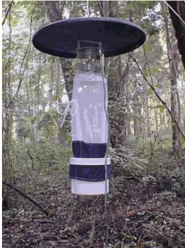
Figure 1. Collection cup fastened to CDC light trap (note the white outer rim securing the cup to the black material)
