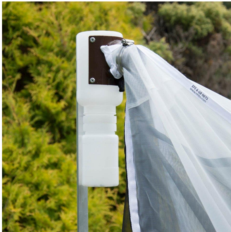
Figure 3. Collection head and attached collection bottle,
