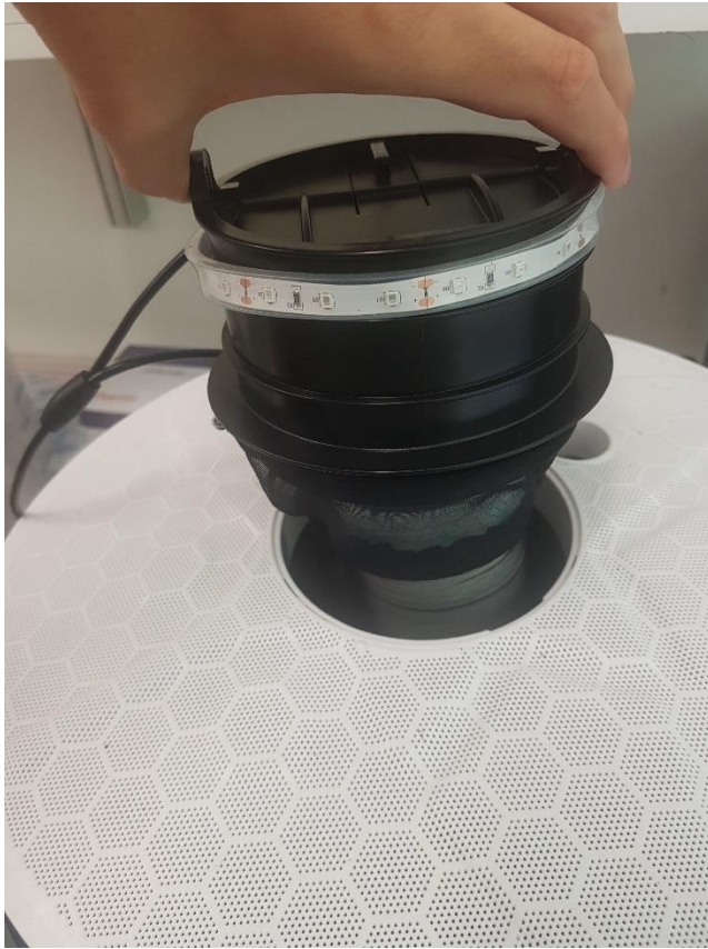
Figure 3. Placing the intake funnel into the trap.
