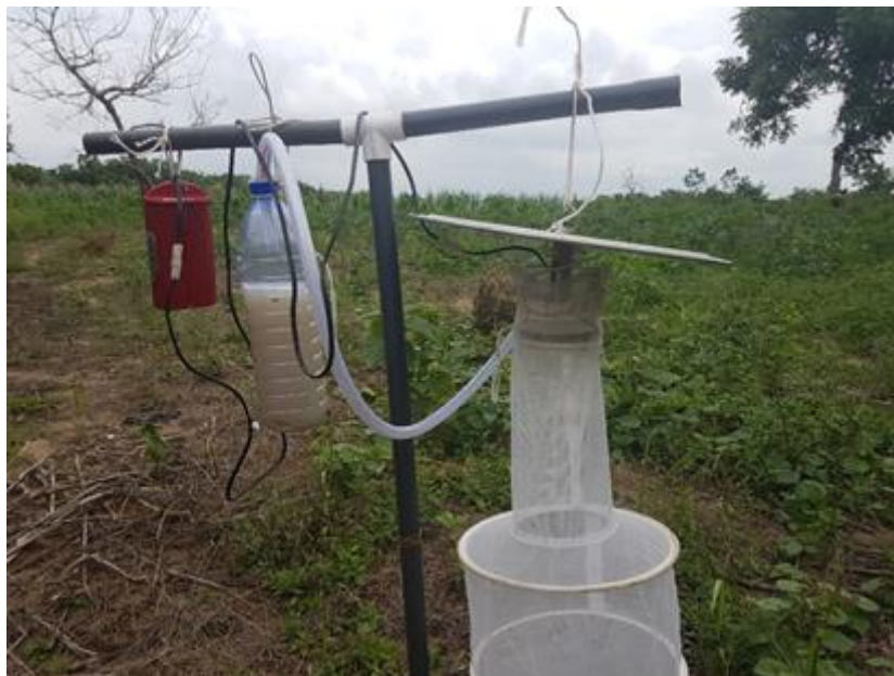
Figure 3. Hose attached to the CDC trap, below the rain protector and next to the light source (note that the light trap pictured will not be the one you use).
