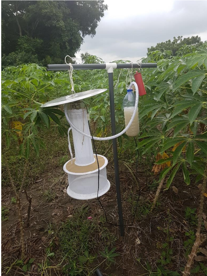
Figure 3. CDC light trap set up. This example uses a net collection chamber and was used only during the first sampling period due to logistical issues limiting the delivery of light traps with ethanol collection chambers. All further sampling was conducted using the ethanol collection chambers traps.
