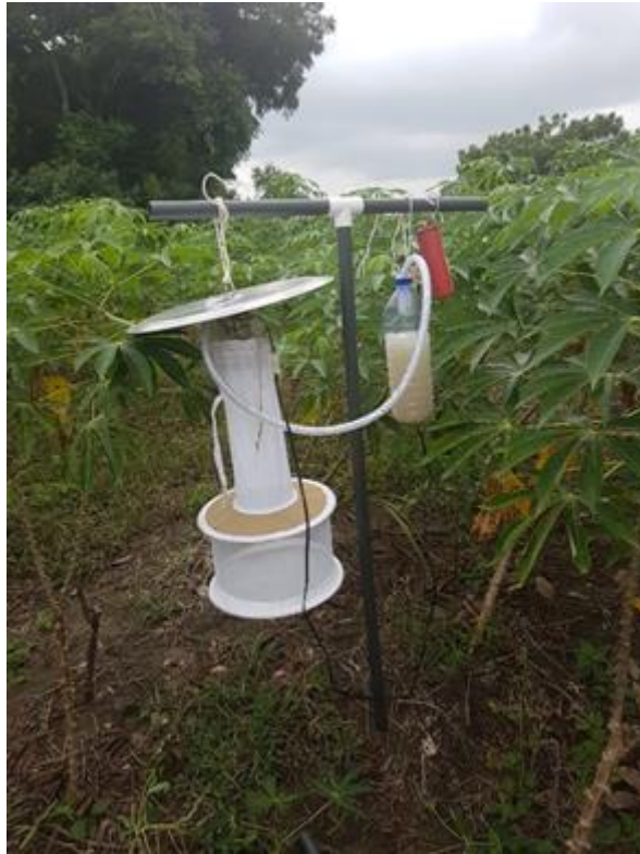
Figure 2. T bar with attached CDC light trap (note that the light trap pictured will not be the one you use)
