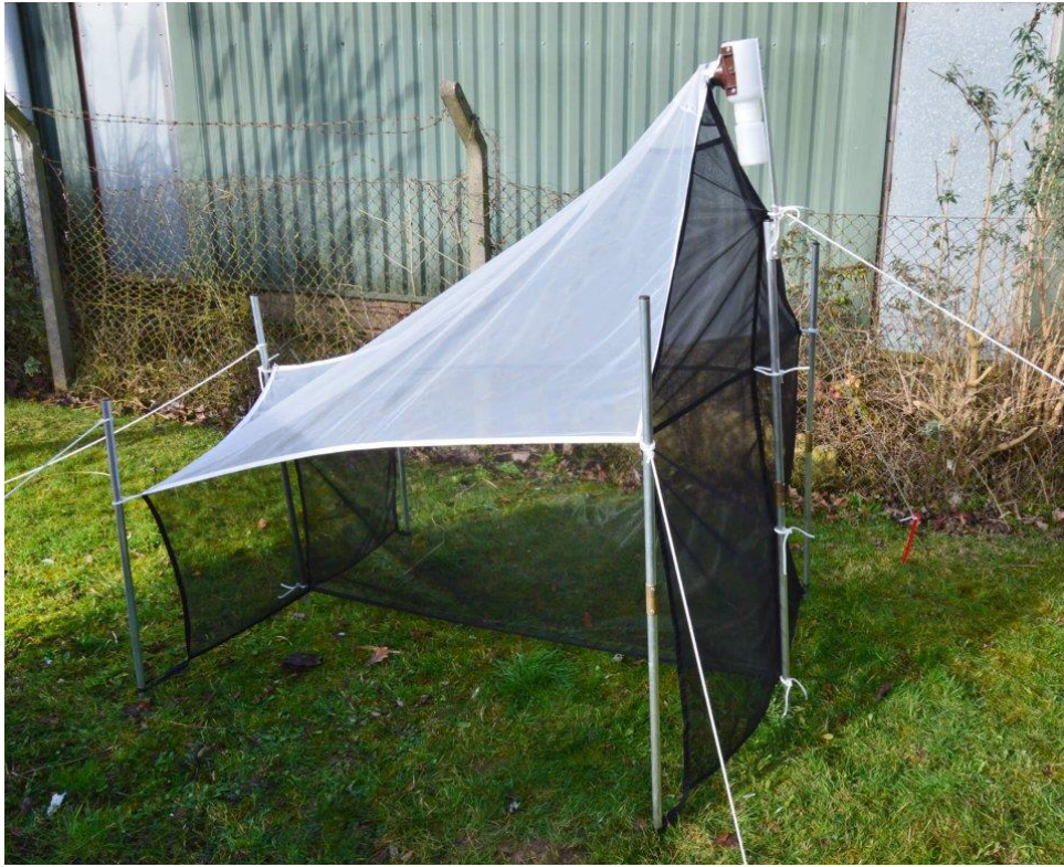
Figure 2. Fully erected trap with taught guy lines.
