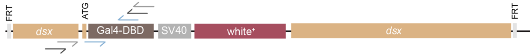
Figure 16 Linear plasmid map of dsx DBD (Pavlou et al., 2016). Brown, grey and blue arrows denote forward and reverse sequencing primer pair locations used in DNA Sanger sequencing verification.
