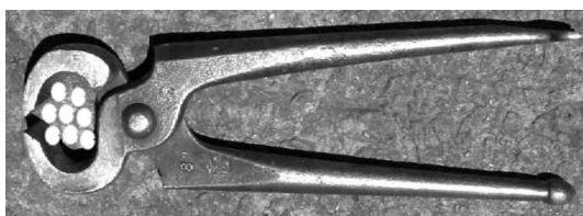
Fig. 13 Each of the two ‘pockets’ in chela of Lardoglyphus zacheri L3 approximates the design of carpenter’s pincers used to grip behind objects (like nails) and then drag them out backwards (image amended under Creative Commons Licence from pincers.jpg by Securiger 23 Feb 2005 https://en.wikipedia.org/wiki/Pliers ). White dots are myofibrils in cross-section, here 3 by 3 being the approximate fixed digit pocket size
