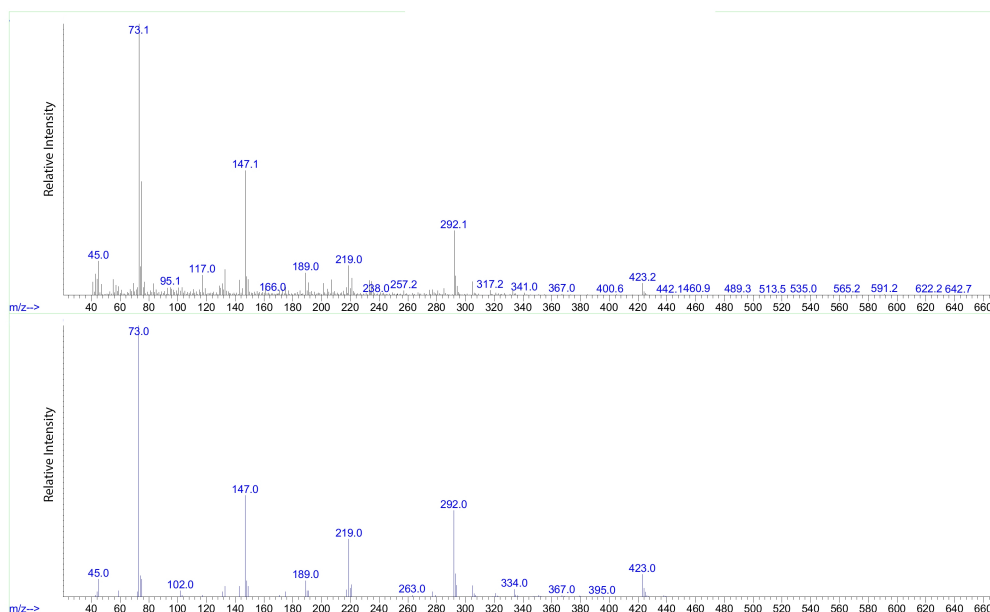
Figure 7.10: Mass spectrum of the peak identified as tartaric acid in Sample BEY006.10622.106 (top) compared against the mass spectrum of tartaric acid (as its trimethylsilyl ester) from the NIST11 database (bottom).
