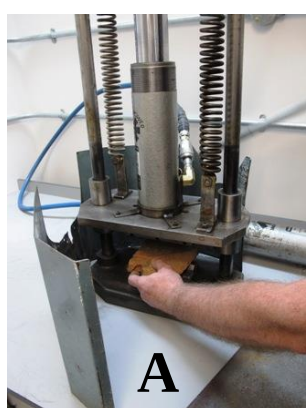
Figure 2-6: A) Rock Splitter, B) Split pieces fed through the grinder, C) Subsequent passes at smaller throat diameters, D) Final >700 \mu m and <700 \mu m.
