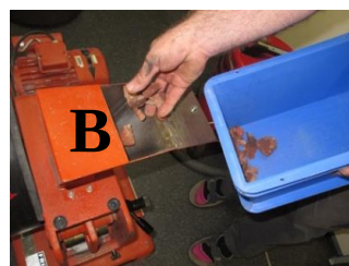
Figure 2-6: A) Rock Splitter, B) Split pieces fed through the grinder, C) Subsequent passes at smaller throat diameters, D) Final >700 \mu m and <700 \mu m.
