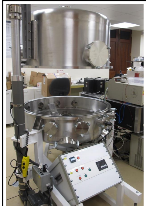
Figure 2-2: Chamber at AOPP that was used to Simulate Mars Environmental Conditions.
