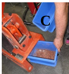
Figure 2-6: A) Rock Splitter, B) Split pieces fed through the grinder, C) Subsequent passes at smaller throat diameters, D) Final >700 \mu m and <700 \mu m.
