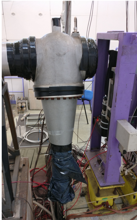
Figure 6.4: The C2 Cherenkov counter installed in the T9 beam test zone. T_b can also be seen on the right within the purple holding mechanics; the scintillator is encased in a black velvet cover, and below extends the single-channel PMT.
