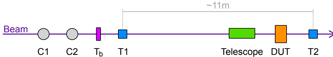
Figure 6.3: The test-beam infrastructure used in the three test-beam campaigns. C1 & C2 are threshold Cherenkov counters, T b a large scintillator, T1 & T2 timing stations, and DUT either Mini-TORCH or Proto-TORCH depending on the test-beam campaign. The position of each item of infrastructure relative to the others is shown, although not to scale.
