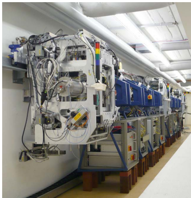
Figure 1: The prototype RTRS after commissioning in the DESY test tunnel (Jan. 2008). The electronics crates in the service cars have temporarily been supported by metal bricks during an analysis of vibration sources.
