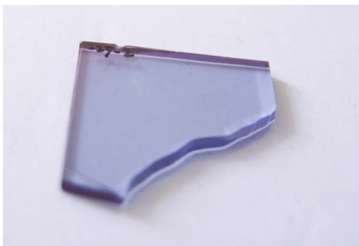
Figure 5.19 Photo showing the appearance of \text{Au/SnO}_2 composite coating deposited on glass at 450^\circ\text{C} using \text{HAuCl}_4 .
