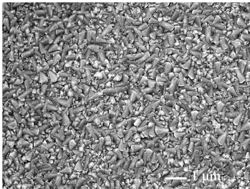
Figure 4.4 SEM image of spray deposited SnO 2 . The scale bar is 1 μm. The film consists of small crystallites with grain size of about 50 nm, along with larger grains of up to 500 nm. The contrast from the crystalline grains indicates a rough surface area.
