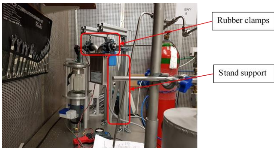
Figure 4.2: Spray rig setup with support and clamps on CFM for external vibration isolation without the aluminium enclosure.
