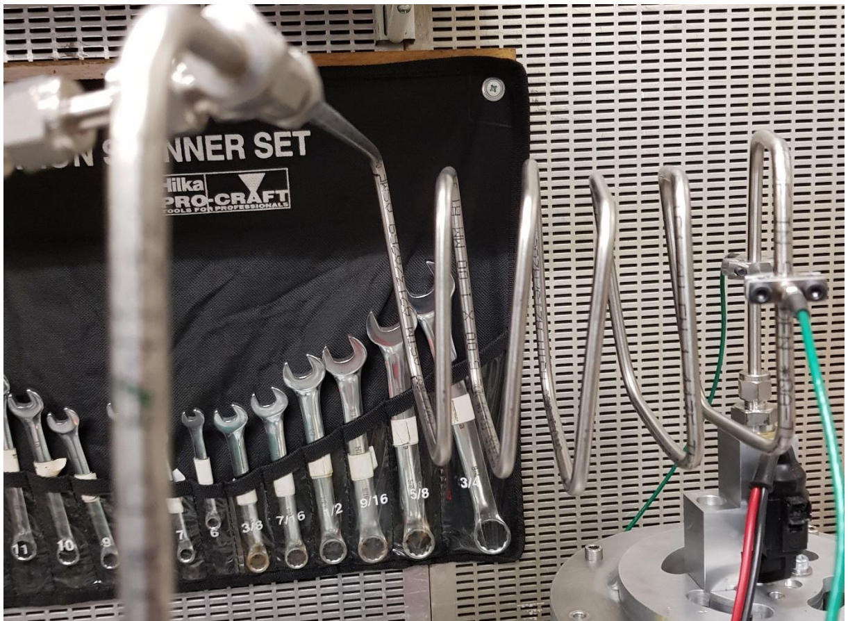
Figure 5.5: Coiled measurement pipeline used in experimental setup 6.
