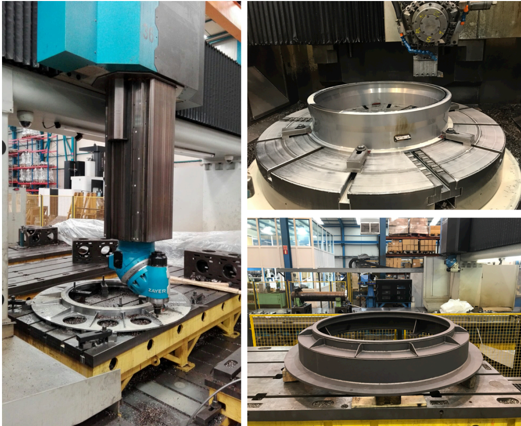
Figure 11. a) Casting die, b) mould and c) machining operation for the design
