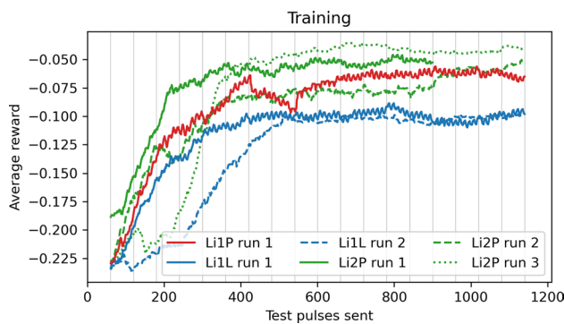
Fig. 7 Average rewards per test pulse sent during the live training on the CRESST setup, smoothed with a moving average of 60 test pulses. Results from six runs with different training settings are shown for Li1P (red), Li1L (blue, blue dashed), and Li2P (green, green dashed, green dotted). For this comparison, we re-calculated the rewards after training with Eq. (2), while during training for some of the runs, the unweighted reward function Eq. (1) was used
