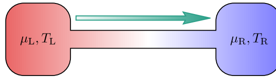
Figure 3.2. Scheme of a system connecting two unequal reservoirs, with temperatures T_L \neq T_R and (or) chemical potentials \mu_L \neq \mu_R . This drives the system to a nonequilibrium configuration, supporting energy and (or) excitation transport.
