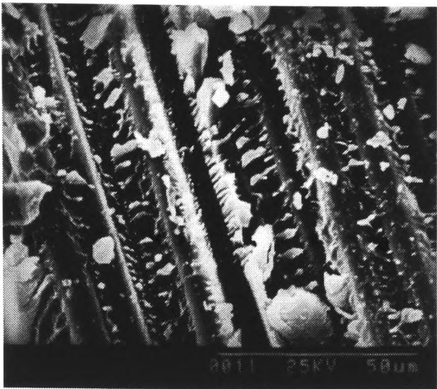
Figure 4.24 CNB3, A Fractograph of Mixed Mode Failure.
