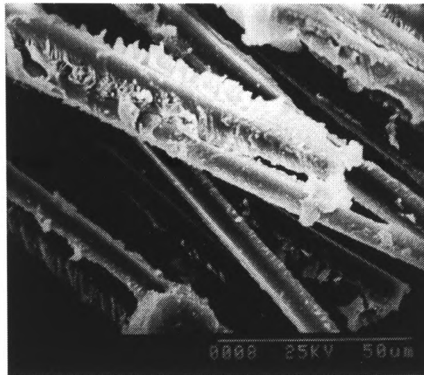
Figure 4.14 IO6, A Fractograph of Matrix Failure due to Pure Shear.
