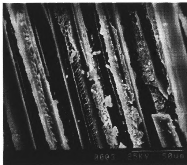
Figure 4.13 IO4, A Fractograph of Matrix Failure due to Pure Shear.
