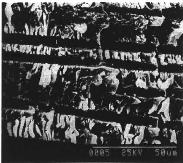
Figure 4.34 PCB3, A Fractograph of Matrix Failure.
