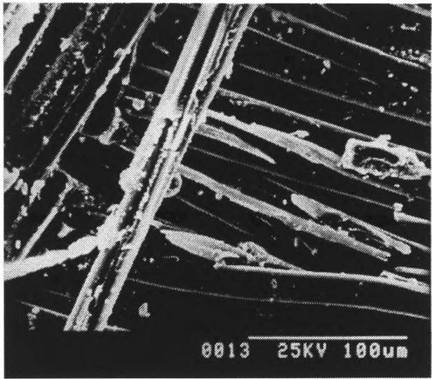
Figure 4.25 CNB4, A Fractograph of Mixed Mode Failure.
