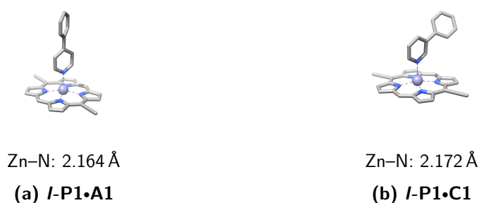
Figure 2.16: Optimised molecular geometries of the host-guest single-site references on B3LYP/6-31G* level. Given values describe the zinc–nitrogen axial coordination bond length.
