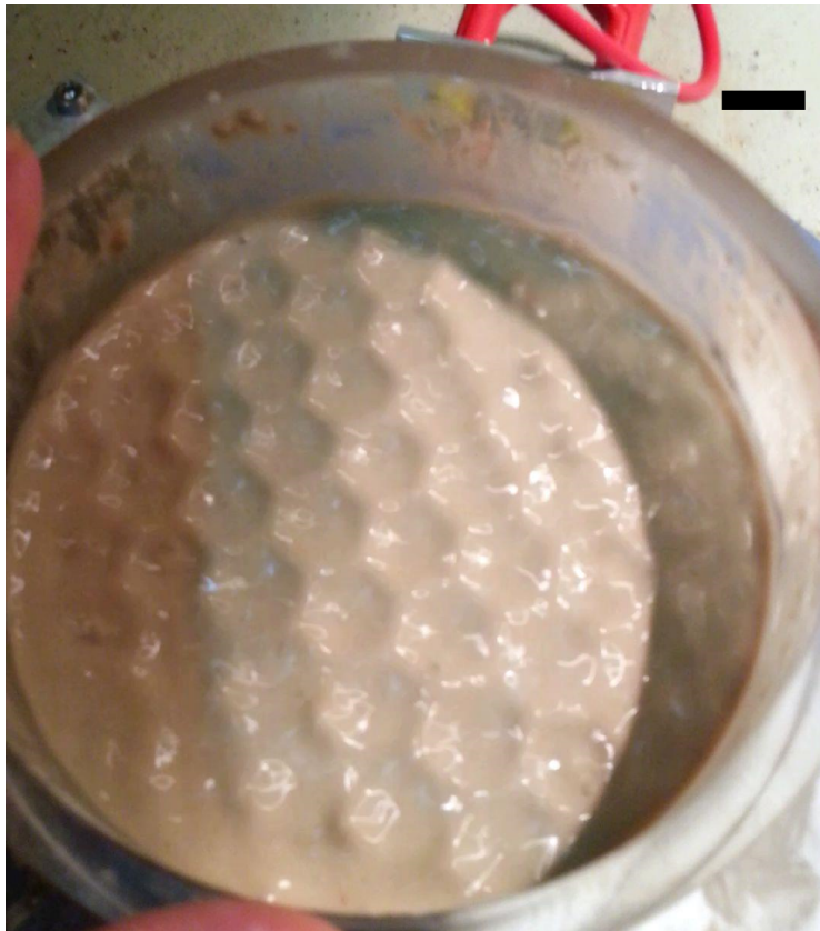
Figure 5.9: Snapshot of an experiment creating a hexagonal Faraday wave mode on the surface of a mixture of two-thirds silica dust and one-third water, with a component of bentonite. Scale bar is 1cm.
