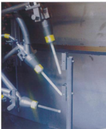
Figure 7.5: Multiple nozzles setup for trials 4 and 5 after (Metal Improvement Company, 2012).
