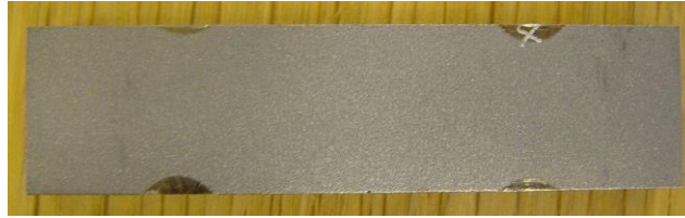
Figure 7.1: Example of the peened test piece after (S.Kennerell, 2012).
