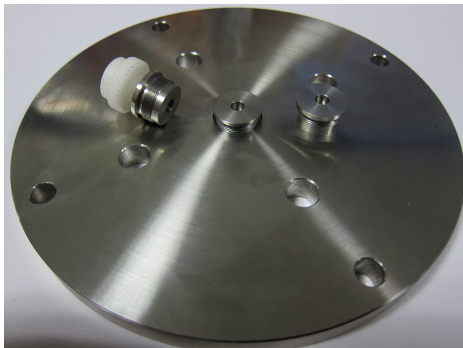
Figure 5.32: Aperture electrode of the ion optic of the new IMS instrument. The central aperture could be removed and replaced with a differently sized one.
