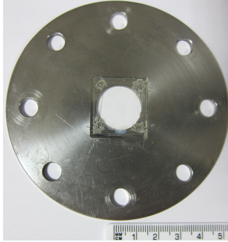
Figure 2.7: Photograph taken of the repeller plate. To load a sample, an ITO coated quartz plate was mounted in the central groove.
