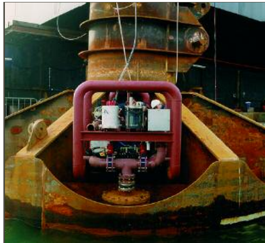
Figure 2.12: Suction pump unit on top of a suction pile (taken from SPT Offshore, http://www.suctionpile.com/pdf/SAPS001.pdf )
