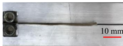
Figure 3.12. DCB specimen in alignment block for nuts bonding with scale bar
