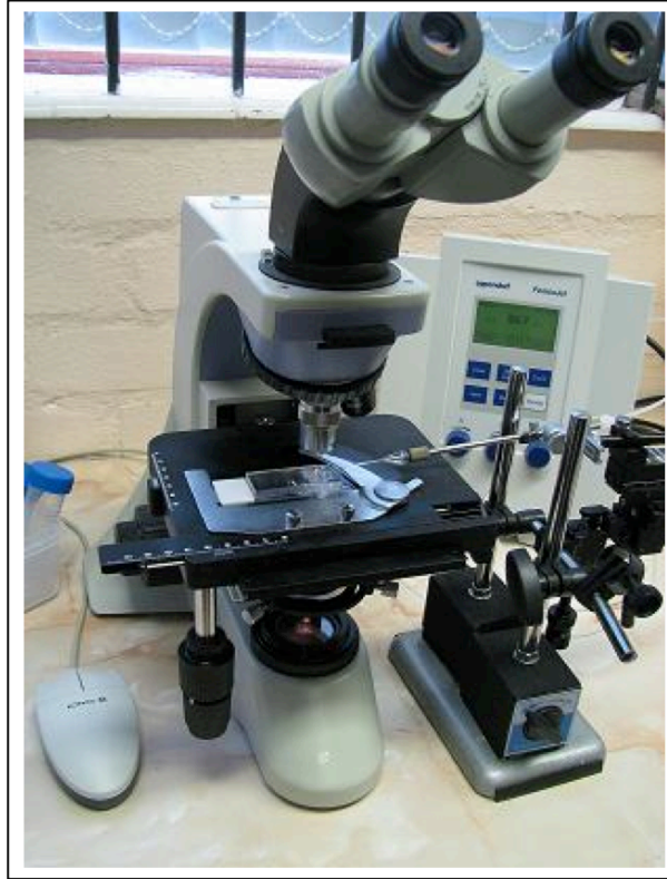
Figure 2.2. Microinjection apparatus. The micromanipulator enables fine adjustments and control of the needle. A constant back-pressure or injection pressure supplied by the microinjector air-pump enables injection of the solution into the embryos.
