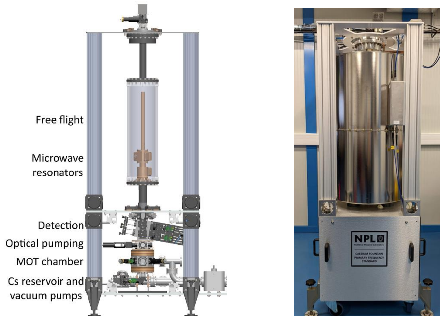
Figure 1. View of the ‘full size’ physics package of the improved NPL Cs fountain design. Left: drawing showing the layout and main functional regions (C-field coil and magnetic shields are not shown). Right: photograph of an assembled unit.
