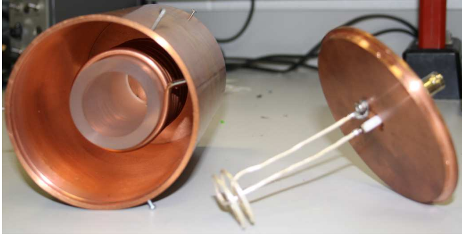
Figure 2.7: Photograph of the helical resonator. The secondary coil is wound around a Rexolite core and enclosed within a cylindrical copper shield. The primary coil is attached to one of the endcaps, and its length iterated to optimise coupling.
