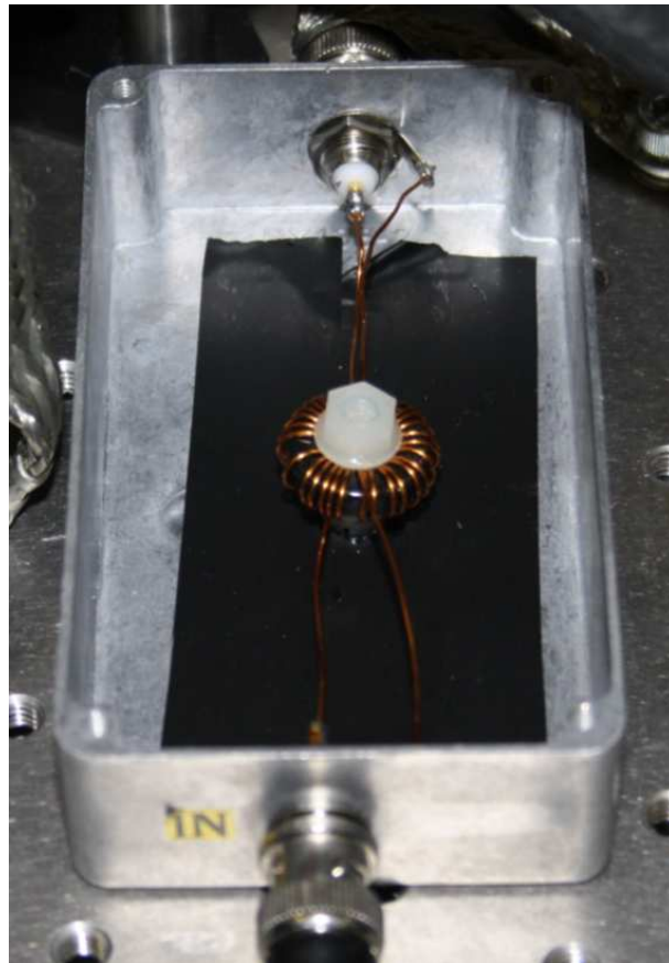
Figure 2.8: In-situ photograph of the toroidal resonator. The core is mounted on a nylon post for mechanical stability.
