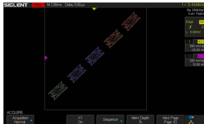
Fig. 24. Attractor self-reproducing in map (1) when d_1 = d_2 = 0 (green is k = 4 ; blue is k = 2 ; purple is k = 0 ; and the last two orange are k = -2, -4 ).
