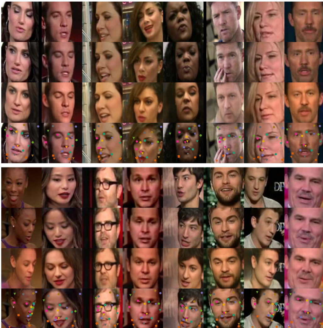
Figure 9: Training with video frames from VoxCeleb. [rows top-bottom]: (1) source image x , (2) target image x' , (3) generated target image \Psi(x, \Phi(x')) , (4) unsupervised landmarks \Phi(x') superimposed on the target image. The landmarks consistently track facial features.
