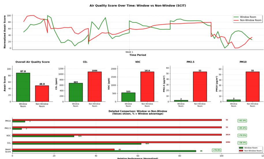
Fig. 3 This figure illustrates the temporal trends of the Awair air quality score, where the green and red lines represent the window and non-window test spaces, respectively. The accompanying bar plots depict the overall density distributions of CO 2 , TVOCs, PM 2.5 , and PM 10 . The plot highlights the advantage of the window test space over the non-window test space in maintaining better air quality across key indicators
