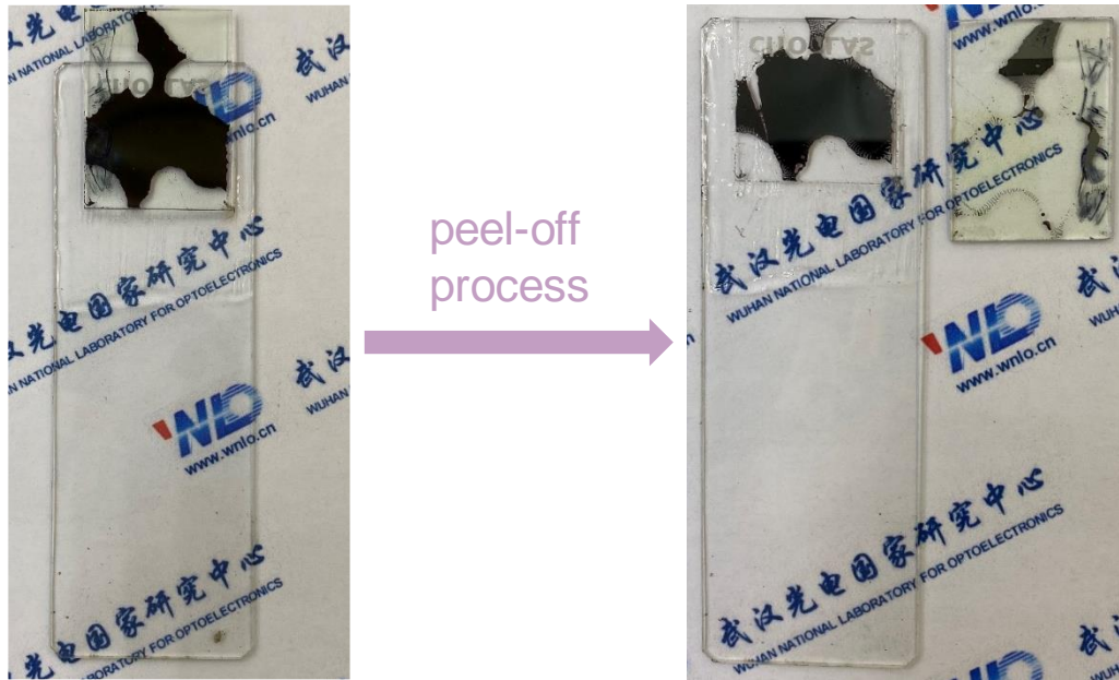
Supplementary Fig. 8. Peel-off method for the bottom surfaces of perovskite films. The bottom surface of perovskite films was fabricated through the following method: the top surface of the prepared perovskite film was partly pasted together with a glass slide using UV glue. After the glue was solidified overnight, the film was peeled off from the ITO substrate with force, and then the bottom surface of perovskite films for characterization was obtained.
