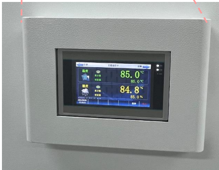
Supplementary Fig. 49. The photographs of the damp-heat chamber in our lab. The temperature and relative humidity levels were maintained at 85 °C and 85% RH, respectively, following the IEC 61215:2016 standard.
