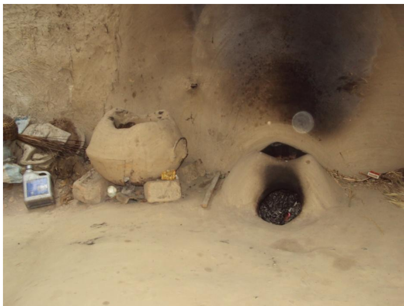
Figure 52: Typical stoves used in the focus group 1 village (for coal – left and for biomass – right) – (photograph by the author)
