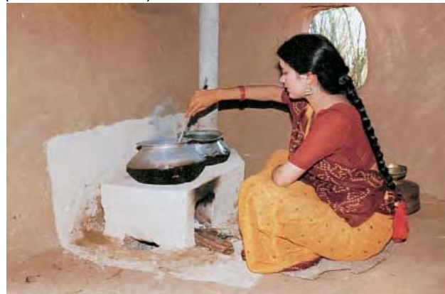
Improved chullah with metal chimney, India (source: (Westhoff et al 1995)
