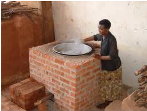
Institutional rocket stove made of bricks (source: bioenergylists.org )
