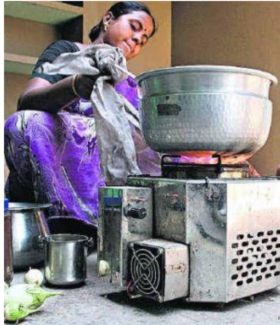
Oorja fan driven efficient pellet stove originally marketed and distributed by BP Emerging Consumer Markets India, now taken over by First Energy Ltd (source: http://biopact.com/2007/07/revolution-in-kitchen-5000-indian-rural.html )
