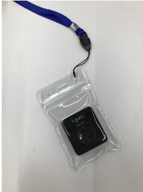
Figure S4.1. GPS logger in waterproof pouch and with attached lanyard.
