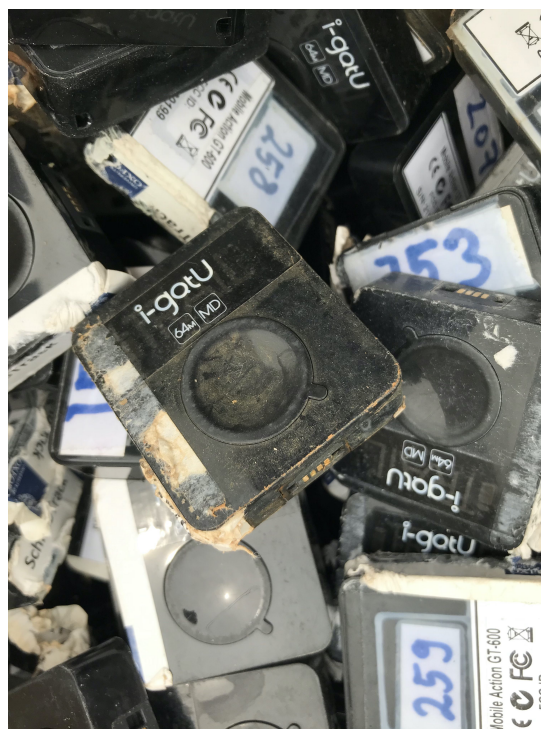
Figure S4.2. GPS loggers with water damage after fieldwork.
