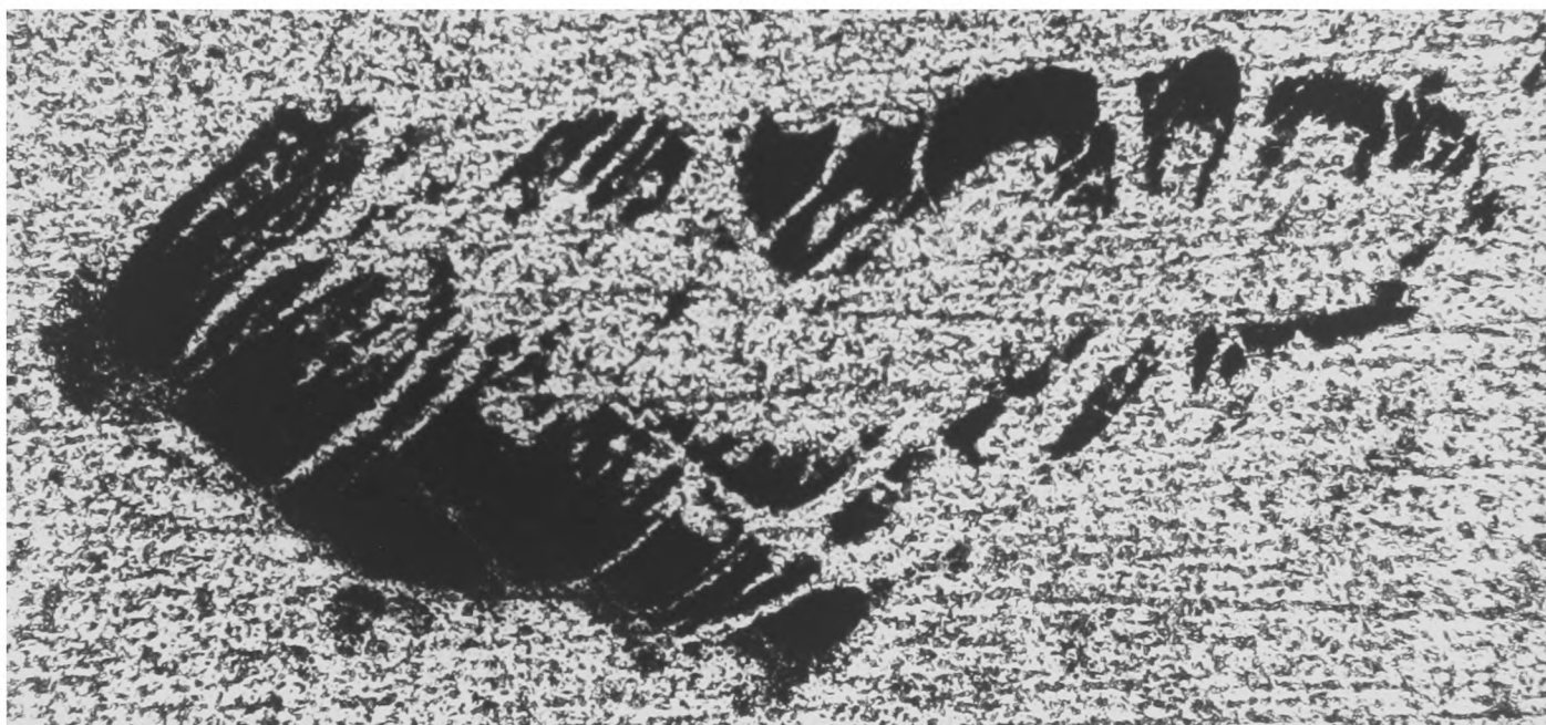
Figure 6.1. Pyroxene bastites rimmed and veined by magnetite. Specimen AG 67.780. Plane polarised light; magnification x10.
