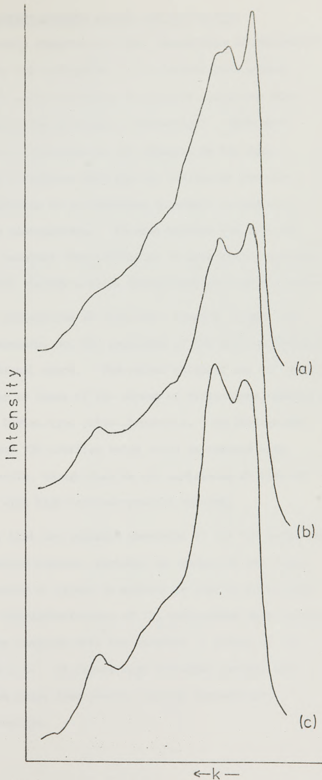
Figure 2.18. Observed profiles of the 130 reflection of chrysotile.
