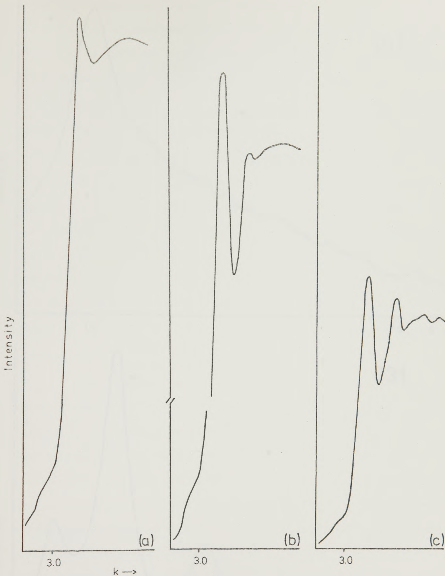
Figure 2.11. Representative weighted profiles calculated for the 031 reflection of helical chrysotile ( N=2 ), for the following values of m_0 and t :
