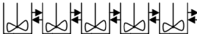
Figure 4.2. Schematic diagram of the cell model with axial dispersion [137].
