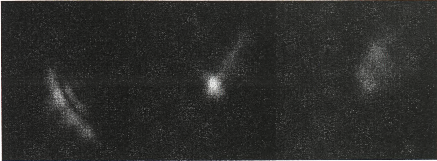
Figure 4-1: Transverse profiles of the laser pulse in the focal region, taken 5 mm before the focal plane (left), at focus (centre) and 5 mm after the focal plane (right).
