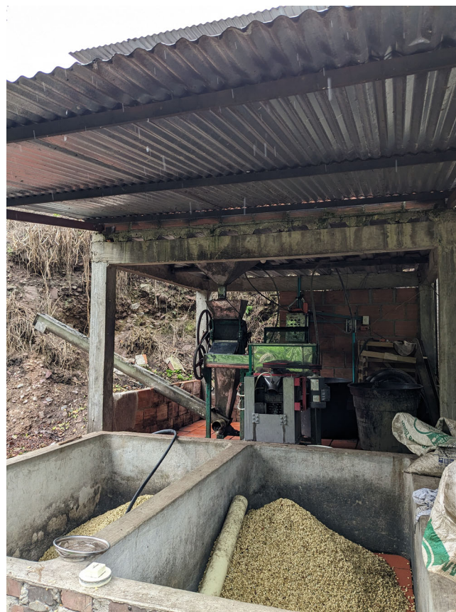
FIGURE 2 A roofed beneficiadero , where harvested coffee cherries are brought for processing, at the Bellavista farm, in a vereda (rural district) of the municipality of Arboledas, Norte de Santander. In the foreground are two cement fosas (basins); in the background, a coffee-pulping machine. (Javier Lezaun and Lina Pinto-García) [This figure appears in color in the online issue]
