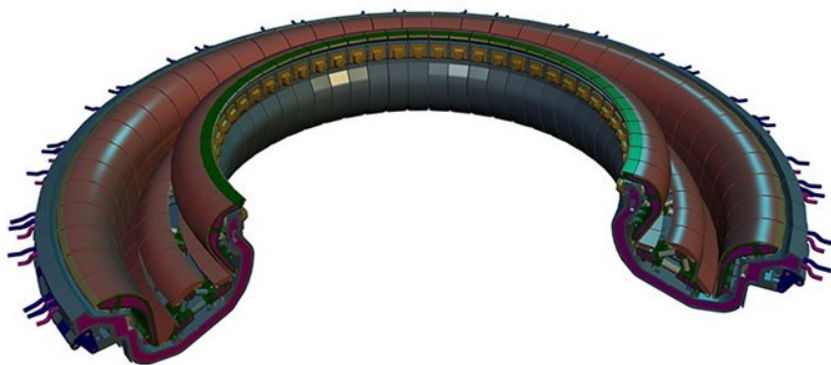
Figure 2.1: Proposed tungsten divertor design for ITER. [12]
