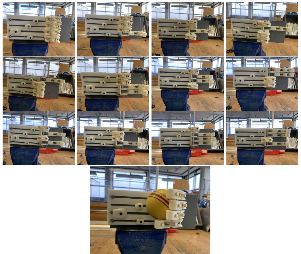
Figure 13. These images show examples of hand gesture combinations executed by selectively locking each of the four fingers, or a combination of these. The final image shows the four fingers holding a sphere when the final position is reached and the air flow has halted. They serve as visual confirmations of the differential and actuation systems' combined functionality.
