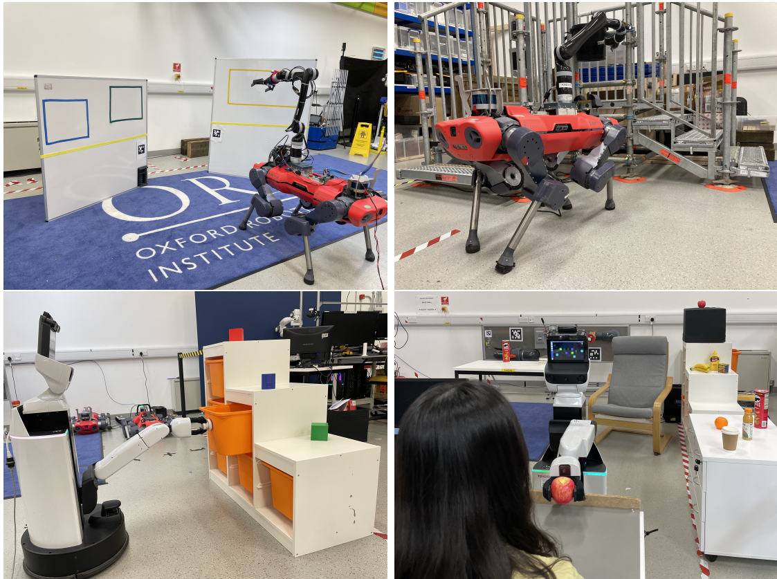
Figure 1.2: Deployment of our TAMP solutions on legged and wheeled mobile manipulators, targeting both industrial and domestic applications.
