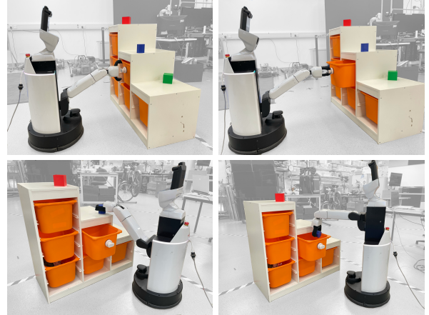
Fig. 1: Physical HSR performing R-LGP solution for table clearing task. The captured actions include grabbing knob, opening/closing drawer, picking object, and dropping object.
