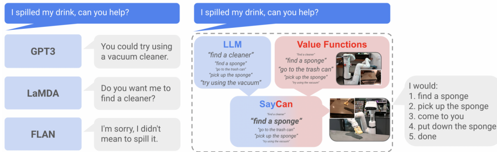
Figure 3.3: While LLMs are not grounded in the world environment, SayCan [111] has been a popular LLM-based robotics planner that considers geometric feasibility during planning with LLM.
