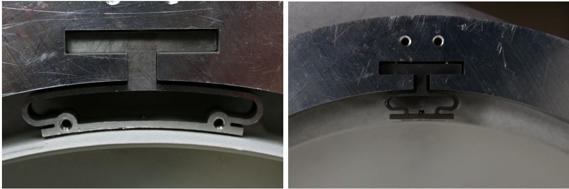
Figure 3.2: Design 1 for the HARMONI spectrograph camera lens mounts using double beam springs for the flexures. Left : version 1 with the longer curved pads. Right : version 2, the current baseline design, with shorter flat pads to make inserting the adhesive easier.
