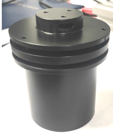
Figure 21. The AmBe calibration source as used in the SNO+ water phase.
