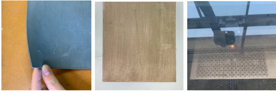
(a) The laserable rubber sheet (b) Sheet coated by metal paint (c) Engraving the rubber sheet
