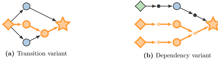
Figure 2.3: As Figure 2.2, but with a possible complete attack highlighted. Note that for the transition variant, the attack is simply a path in the graph. For the dependency variant, the attack cannot be represented as a path.
