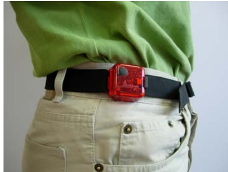
Figure 15: Photograph demonstrating correct positioning of accelerometer
