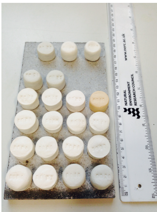
FIGURE 6.1: \sim 10 g Kaolin and montmorillonite clay standards fired at 825^\circ\text{C} for 7 hours. The samples are stamped with a reference number to aid identification.
