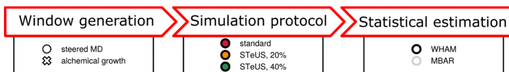
Figure 3. The three steps of an umbrella sampling study, and the individual components compared in this work. The nomenclature defined here is used consistently throughout Figures 4, 5, 6, 7, and 8. Window generation methods are distinguished through shape, simulation protocols through fill color, and the use of temperature reweighting (MBAR) or ground-state information only (WHAM) with the outline color.
