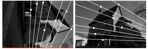
Figure 11: Example epipolar lines and correspondences using the computed fundamental matrix.
