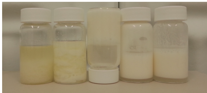
Figure 5.2: Photograph of emulsions stabilised by TA-PVP particles. The oil volume fraction ( \phi_{oil} ) varies from 0.82, to 0.74, 0.60, 0.50, 0.30 left to right. The vial in the middle is at \phi_{oil} 0.60 and it is upside down to better show the resistance to flow of this emulsion.
